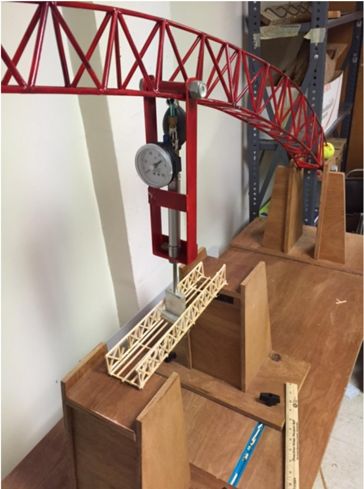
The Bridge Testing Apparatus
